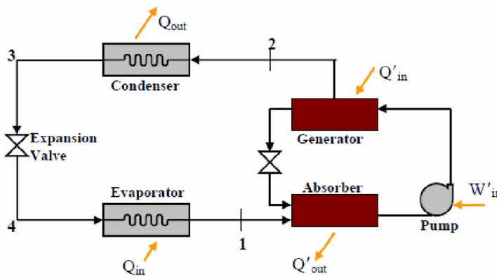
Figure 2: Absorption Chiller Schematic
