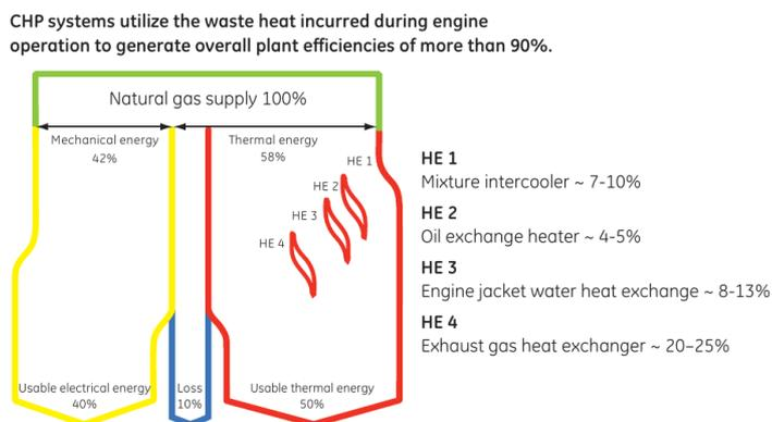
Figure 3: Sankey Diagram of energy flows in a GE reciprocating gas engine. Source: [http://site.ge-energy.com/prod\\_serv/products/tech\\_docs/en/downloads/GER3430G.pdf](http://site.ge-energy.com/prod_serv/products/tech_docs/en/downloads/GER3430G.pdf)
