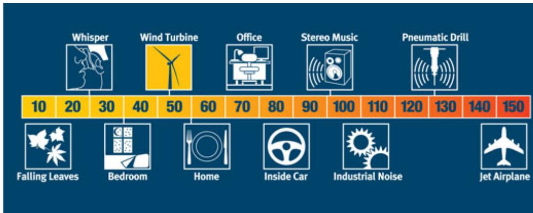
Figure 1: Sound pressure levels of wind turbine compared to other common sources ([www.canwea.ca/wind-energy/myths\\_e.php](http://www.canwea.ca/wind-energy/myths_e.php))
